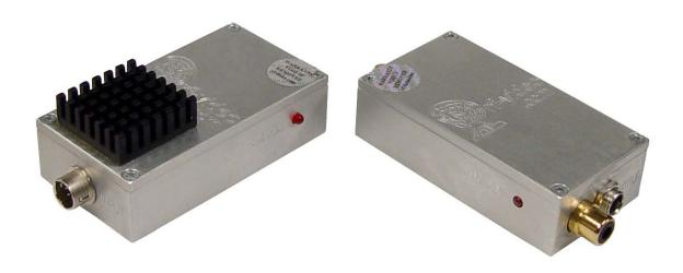
New Microwave Transmitter and Receiver are fully synthesized single channel items (5,644.750 MHz). The RF power output power is 200 mW. They are great for low range communication up to 2500 ft LOS or experiments.
