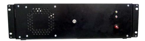
Model AVX-50/UHF is a new professional TV linear amplifier in A class with 50 W RF output power and only 4 W input power. This amplifier is using latest technology with built-in switching power supply. It is light (weights only 10 lbs) unit. This amplifier is recommended as a driver for high power stages or small TV stations.
